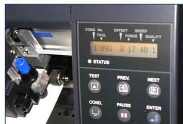
**Step 8:** Using the arrows on the Qe-60+ control panel, move the cutting head so that it's over the lower right hand registration mark. Push the Origin button to set that as the new origin point.
