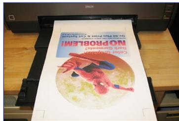
**Step 6:** Load the paper in Qe-60+. Select Sheet from the Load Media menu. Position the pinch rollers on the edges of the media. To reduce skew, use the strakes on the front of the plotter platen as guides.
