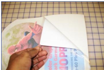
**Step 18:** Place the weeded, masked graphic on your garment of choice on a heat press capable of producing 350°F. We are using a Knight DK20-AR clamshell press with an advanced auto release feature.
