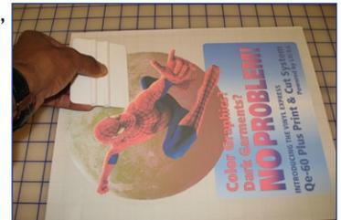
**Step 17:** Pull the tape upward (or flip the graphic over and gently remove the liner by pulling it away from the masked graphic). Now your masked graphic is ready for the heat press.
