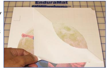
**Step 15:** Mask the weeded graphic using a high tack transfer tape. This will become the liner for applying the graphic to the garment on the heat press. Siser ColorMask works particularly well.
